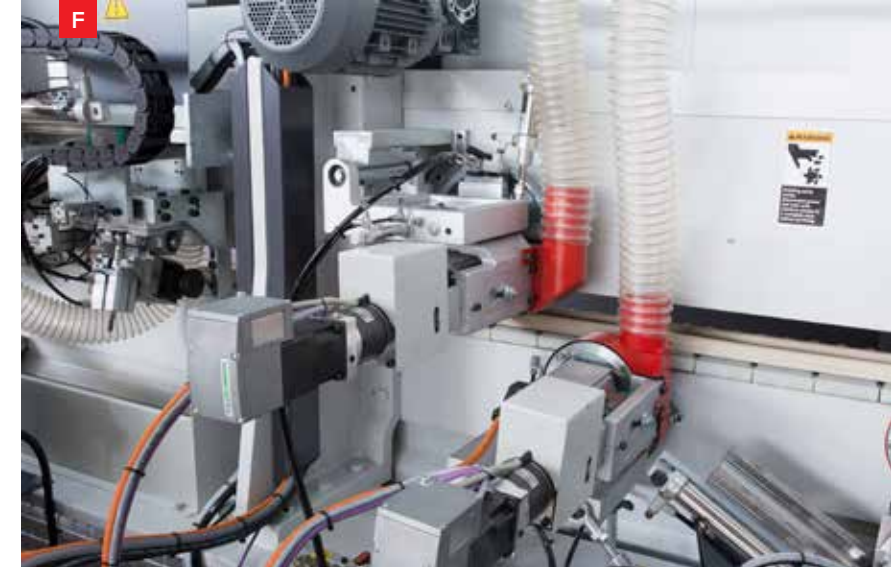
F Servo Kontrol Bant Geçiş Sistemi / OPSİYONEL Band Transition System With Servo Control / OPTIONAL
